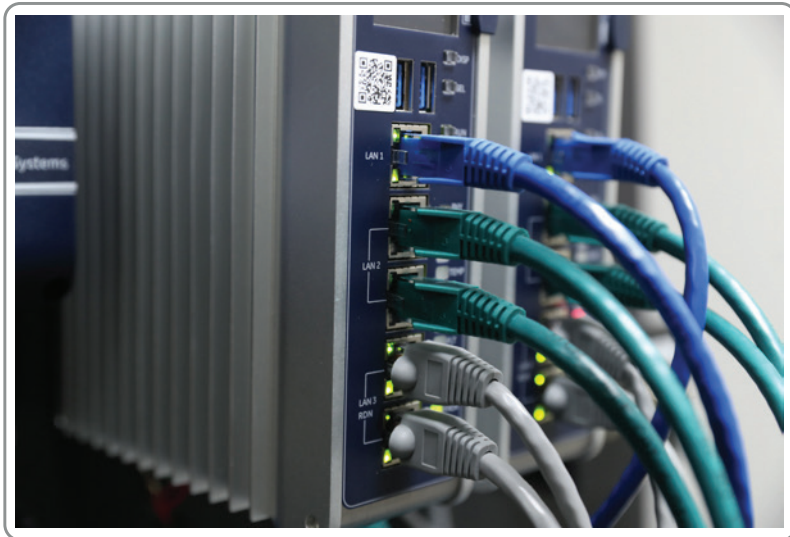
Figure 4. Edge controllers feature multiple cores managed through carefully designed virtual machines (VMs) and provide a unique combination of deterministic control like a PLC or PAC, and independent general-purpose processing like a PC.
