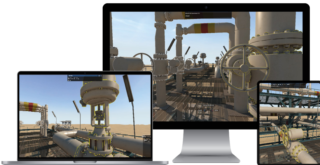
Figure 1. Dynamic simulation can be used to train operators and test control strategies in the control room or even in the field.
